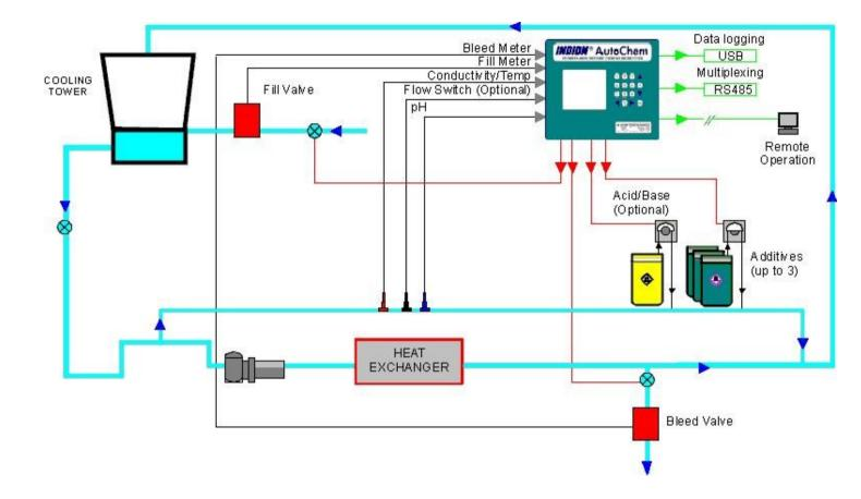
A representative diagram of INDION AutoChem installed in a conventional evaporative cooling tower system
